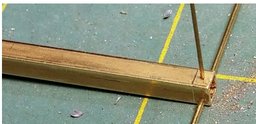
Figure 8: The universal end of the square shaft was made in a similar manner as the sleeve coupling. Here is a finished vertical hole of 0.020" in diameter with a horizontal hole of 0.032". Both holes extend through both walls of the square tube. The scribed line marking the finished width of the piece is visible in the photo.
