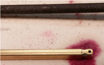
Figure 5: Using a rat tail file the square sides of the tube were rounded slightly on both sides of the hole.
