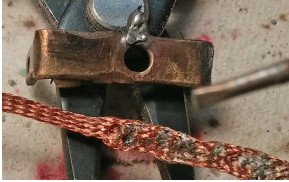
Figure 21: De-soldering braid and my soldering iron were employed to wick off excess solder that remained on the truck frames.
