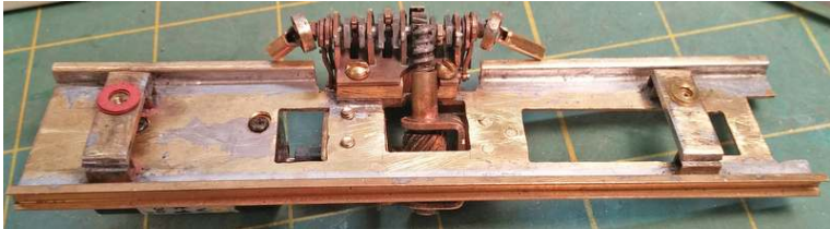
Figure 23: Here the phosphor-bronze wire is shown trimmed to length and bent against the two insulated wheels on a truck. A piece of 30 gauge stranded wire provides a current path to the grounding lug on the frame in addition to the path provided by the truck's mounting screw.
