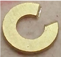
Figure 26: A segment was cut out of a 2-56 washer using a pair of rail nippers.
