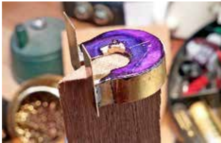
Figure 168: A scrap of wood was used to support the 0.010" brass of the backhead while marking hole centers. Here a portion of the oil fire door has been removed to allow for the electric motor's drive shaft.
