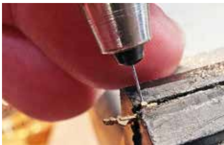
Figure 170: This is the oil firing control and it needs a rod extending from its bottom side through the deck of the cab. Linked by this rod to a valve on the oil line leading from the tender this item controls the flow of oil to the firebox. The hole center was dimpled with an awl and drilled with a #79 bit.
