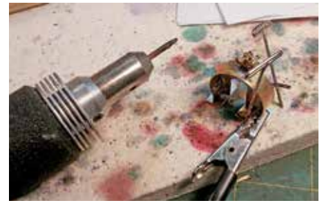
Figure 173: This photo was taken seconds after soldering the steam turret to the backhead. The joint was achieved almost instantaneously. However, the weight of the grounding clip and its wire made the backhead, being such a small part, very difficult to control.
