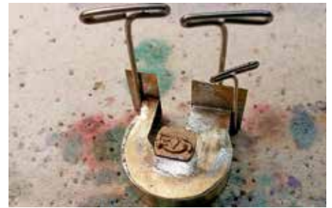
Figure 167: The oil fire door was the first part soldered to this assembly. It was the one part that could safely be placed first on the backhead. The door had to be cut after installation to match the U-shaped hole for the electric motor's drive shaft. This was done with a jeweler's saw and round file.
