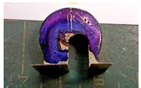
Figure 169: It seemed best to mark and drill all the holes I could before adding more parts. Drilling holes after soldering parts on could be a risk to those parts. One hole could not be drilled, however, as its location depended upon two adjacent parts for its placement. Shown are the holes for the backhead throttle and the three petcocks.
