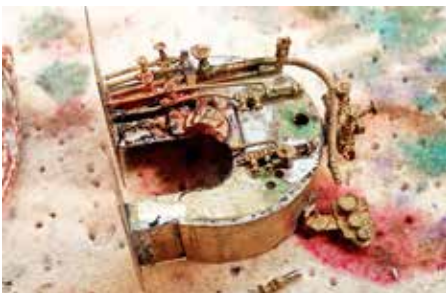
Figure 178: One of the petcocks has been installed in the first of three holes. The second one is in the foreground of the photo.
