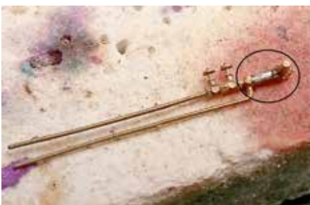
Figure 176: This is one of the two water glasses in the backhead kit. At the right is a small section of the part that has been tinned. The mounting stud is at the far right end of the part.
