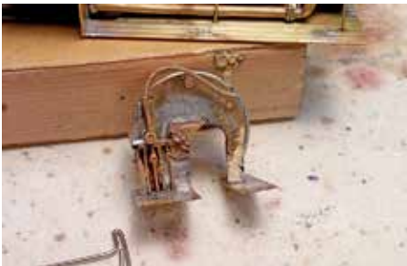
Figure 174: The backhead is taking shape. The oil burner valve cluster is on the left. The predrilled holes mark locations for other parts.
