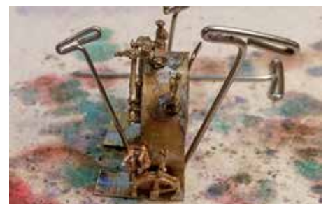
Figure 179: I had to remove the air controls and then solder the reverser quadrant into place. Then I was able to reattach the air controls. I should have installed them in the reverse order of what I originally did.
