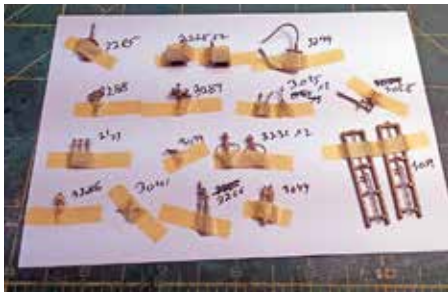
Figure 166: All the parts of the backhead kit were taped to a file card and labeled for ease of identification during assemble. These are from Precision Scale's Backhead Detailing kit for 50-70 oil burning Shays. (#3719)
