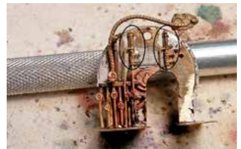
Figure 177: Both of the water glasses have been attached in this photo. The small pipes running to the cab's deck have been removed from the one on the right because of the drive shaft opening.
