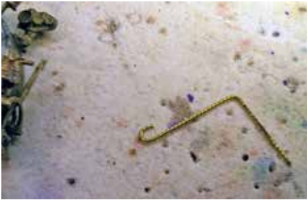
Figure 180: I used a #79 drill to clean out the hole that came in this 2 ½” globe valve from PSC. Once this was done a piece of 0.012” brass rod slid easily through the part. Once that rod was soldered into the valve the large sprue at the bottom of the part was removed.
