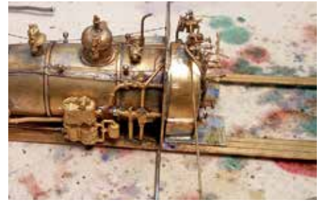
Figure 181: This is a trial assembly of the backhead with the rear of the boiler and it was done to mark the spot where a steam line from the turret runs through the cab front to the air pump.
