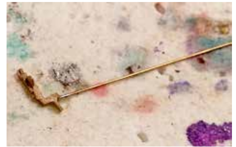
Figure 175: Here a 0.012" brass rod is soldered to the oil firing control before being attached to the backhead. In a real Shay that rod would link the control to an oil valve beneath the deck of the cab.
