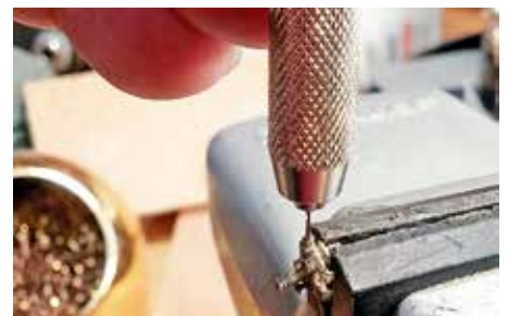
Figure 171: Some parts come with their hole centers marked with a dimple or a cup molded into the part as does this steam turret. While the cups need not be drilled deeper I find they will hold their associated pipes more securely if drilled out prior to soldering.
