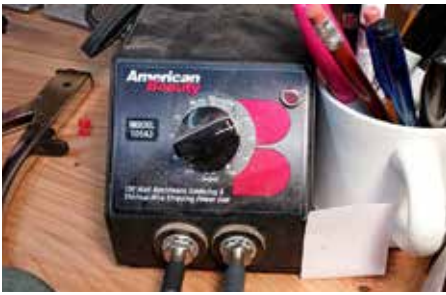
Figure 172: This is my resistance soldering unit. It has two interchangeable leads seen coming from the front of the unit. One lead powers the electrode while the other is attached to the grounding clip.
