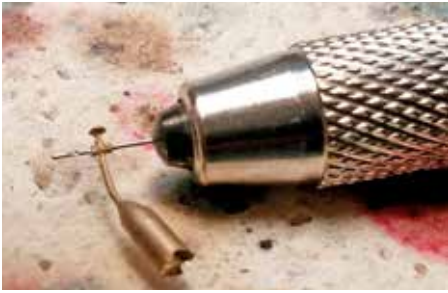
Figure 180: I used a #79 drill to clean out the hole that came in this 2 ½” globe valve from PSC. Once this was done a piece of 0.012” brass rod slid easily through the part. Once that rod was soldered into the valve the large sprue at the bottom of the part was removed.
