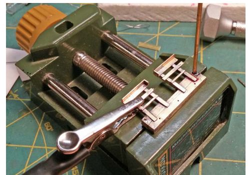
Figure 47: 1/16" diameter brass tubing was soldered over the centering pins made in the last step. The tubing was then cut and filed to length. Finally, the open end of the tube was drilled with a #55 drill to create the contour of the pole pocket.
