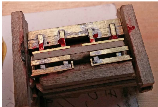
Figure 45: The same fixture was used to hold the horizontal braces on the floor board hangers in place while being soldered. Scale lumber was used to accurately space the parts. The horizontal braces were then cut and filed to length.
