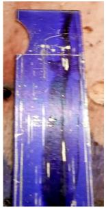
Figure 105: Shown here is the engine shroud while still a flat piece of brass. The curved cutout matches the diameter of the boiler and was traced from one of the card stock patterns made during installment 10 of this series.
