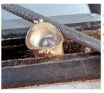
Figure 115: The sand dome was sloped, but naturally it did not match the slope of my boiler. I adjusted its slope with a wide oval shaped file and then finished matching the curves with sand paper as I did with the smoke stack. The sand dome is Precision Scale Company # 32385.
