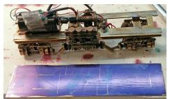
Figure 101: The underside of the deck was scribed to mark the cutouts needed to accommodate the frame, motor, gear tower, and the engine. When doing something like this, remember that you are creating a mirror image of what is seen on the top of the frame; I didn't the first time.
