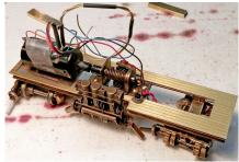
Figure 103: The deck in place on top of the frame. Though not shown in this photo, the end beams were installed at this point to ensure that the deck aligned with them properly.
