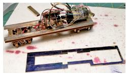
Figure 102: The underside of the deck is shown here. The edges of the cuts were smoothed with a flat jeweler's file. Whenever smoothing out long cuts such as these, keep as much of the file in contact with the edge as possible; this will create an "average ride" for the file and smooth the edge more evenly.
