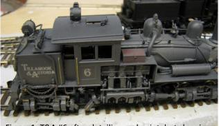
Figure 1: T&A #6 after detailing and paint, but showing a broken universal coupling on the aft drive shaft.
