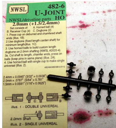
Figure 18: This is the universal joint used in Shay #6. Note the short dogbones to the left of the part sprue. Their length and the shaft diameters must be selected for the particular application at hand. Part #482-6 was perfect for the cramped space inside the tender of the new Shay #6.
