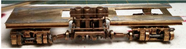
Figure 14: The trial assembly of the frame, engine, and trucks. The worm on the engine was turned by hand at this point to determine that the gears, universals, and trucks operated smoothly and without binding.
