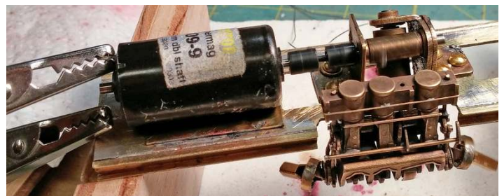
Figure 19: The gear train of #6 running smoothly under power as shown by the blurred worm gear near the center of the photo. It ran smoothly in both directions and was
