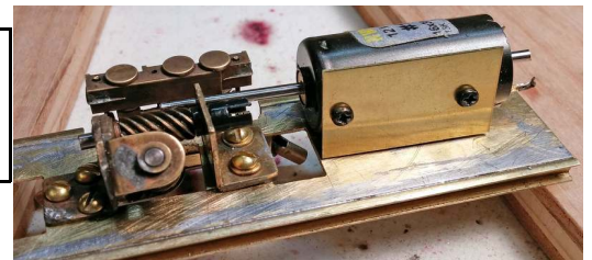
Figure 17: The new can motor for Shay #6 as attached to its mounting plate. Clearance holes for the screw heads were drilled in the loco's deck before the plate
