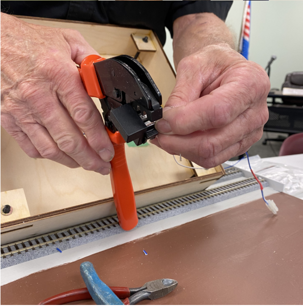
(above) Lloyd Horst crimps a Powerpole connection with a Powerworx crimp tool. Note the Kato connector is also available if needed.
