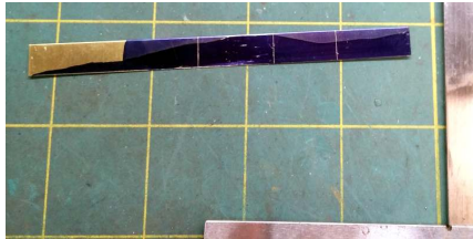
Figure 53: A strip of 0.010" brass swabbed with Dykem and the dimensions of the three sides of the firebox were scribed onto it.
