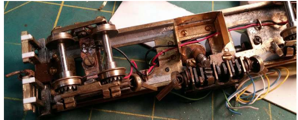
Figure 60: This is a trial assembly of the firebox and ash pan to the underframe of #6. The part was then removed for adding detail and to make the addition of the truss rods easier (coming in part 8 of this series).
