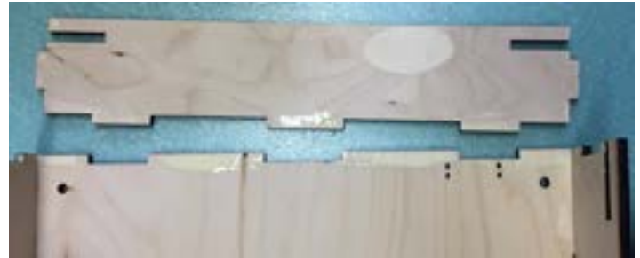
Figure 3: After applying wood glue to the tabs, each piece easily slid into place.
