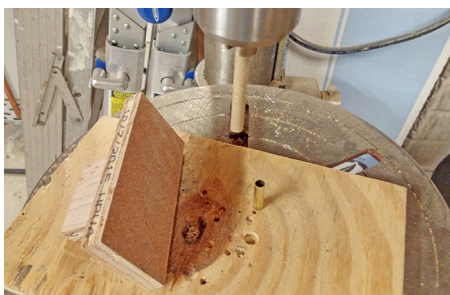
Figure 139: Shown is a length of poplar dowel chucked in my drill press. Below it is the 1/4" brass tube that will become the body of the tank. My sanding block, on the left was made by gluing two pieces of birch plywood together and then I glued a piece of 150 grit sand paper to the face of the larger block. Franklin Tightbond II was used in both cases.
