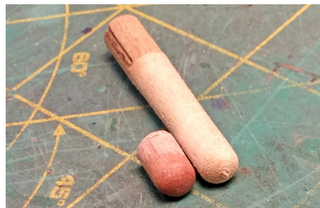
Figure 140: Two pieces of dowel are shown with their ends rounded. The end grain on the rounded surface was very porous looking (shown on the right) so I put a drop of Dr. Mike's Model-n' Crafter's Glue on the end. This wicked right into the wood grain sealing and filling it nicely. In a few minutes I used a piece of 800 grit sand paper to smooth the rounded end of the left dowel.
