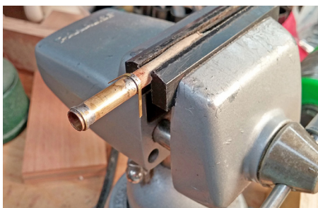
Figure 141: The length of the .015 x .042 brass strips was determined to be .785" by using the formula Circumference = \pi d . The strips were measured and marked using a micrometer as described in an earlier installment of this series.
