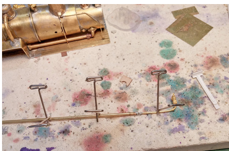
Figure 135: The full length of 1/16" brass tube and the right side check valve were pinned in place before soldering. The second half of the coupler joint was made with Rickety Rails detail solder.
