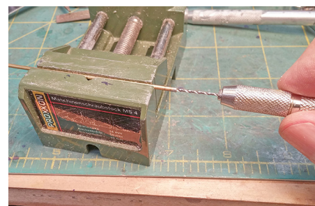
Figure 134: Here the end of a piece of 1/16” brass tube is being drilled out with a #65 drill. It was only drilled far enough to create a secure seat for the pipe from the right side check valve.
