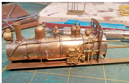
Figure 133: The Worthington air pump (Cary # 13-667) was soldered to the boiler from the inside. The pump, fortunately, covers the end to end solder joint between the injector and the check valve.
