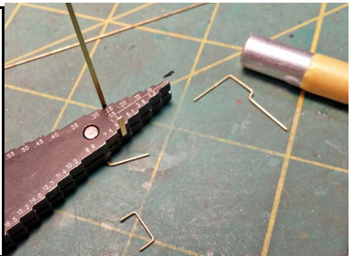
Figure 84: Here a lever carrier is partially formed using my Grabhandler.
