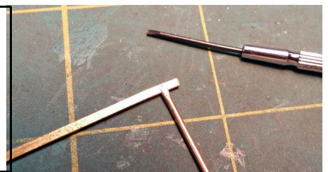
Figure 80: A clevis shown in the process of fitting around a piece of 1/32" x 1/64" brass.
