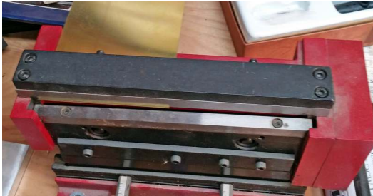
Figure 83: Several narrow strips of brass were cut off of a piece of 0.010" brass sheet for the lever carriers.
