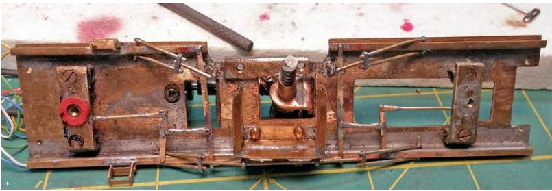
Figure 82: The brake levers, clevises, and rods shown in place.
