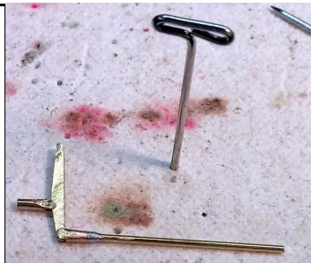
Figure 81: An intermediate lever assembly shown with two clevises. The short piece of 0.032" diameter rod soldered into the bottom clevis runs to the centerline of the trucks.
