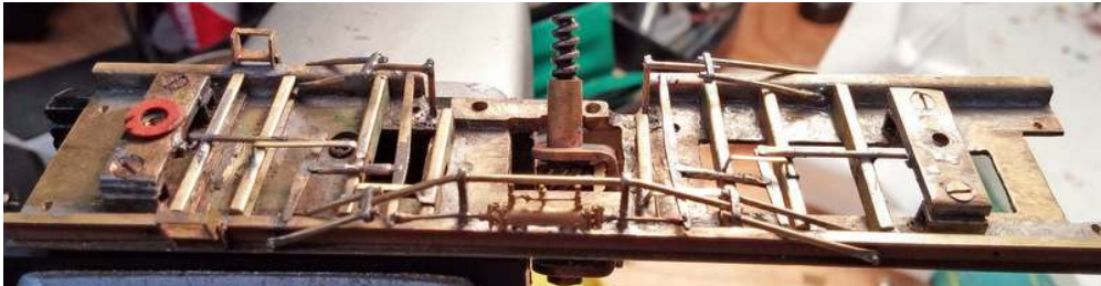
Figure 86: Channels added as support for components after the brake levers and rods were in place. The four lever carriers are now mounted on these beams.
