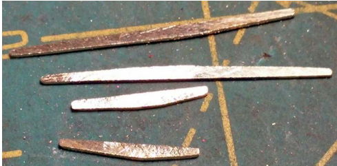
Figure 77: The two cylinder levers shown here with the two intermediate levers needed for Shay #6.
