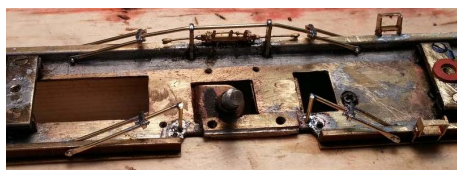
Figure 75: The dummy truss posts that will be hidden behind the cylinders. These were just 0.032" brass rod soldered into holes drilled in the frame. They are shorter than the posts they replaced and were used to achieve a better angle on the right side truss rods.
