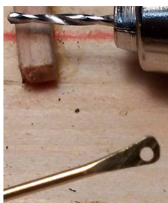
Figure 71: This is a finished truss rod end. Here the end is shown after the hole was cleaned up with a small reamer. A total of 8 are required.
