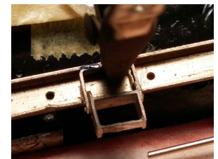
Figure 68: An alligator clip holds a step in place for soldering. The two holes in the side channel are for the rear end beam support and the right truss rod ends
