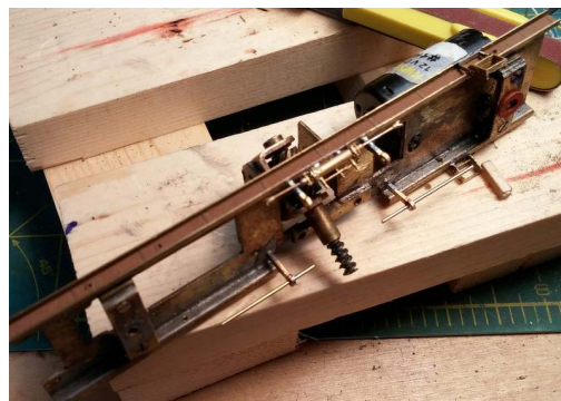
Figure 70: Here the left side channel detail is glued in place. Note the rivets and gusset plates on the part. These are actually scale size.
