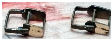
Figure 67: The Shay steps used were Precision Scale #HO-3125. The one on the left shows the notch which was cut into them so they would fit over the frame's side channel.
