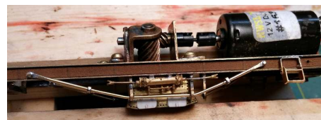
Figure 76: This shows the left side of the new #6 with the firebox and ash pan reinstalled. The steam jam sits between the truss posts.
