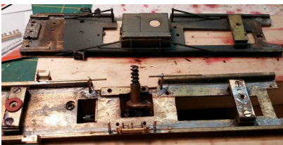
Figure 66: Putting square pegs into round holes. The image above compares placement of the truss rod posts on the old and new Shays #6. Note the steeper angle of the right truss rod on the older version. The steam jam shown is a Precision Scale Company #HO-3101.
