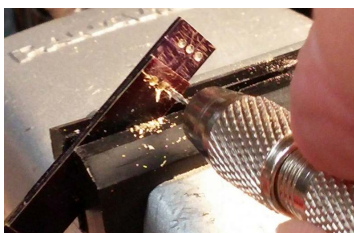
Figure 73: The truss head template and a #65 drill bit were used to mark the hole centers for the required four truss heads before they were piloted with a #76 drill.
