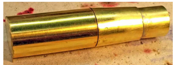
Figure 99: The completed boiler and smoke box assembly. The boiler head seen at the right will be notched to accept the drive shaft running from the motor to the gear tower.
