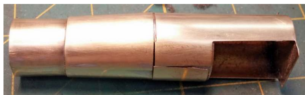
Figure 100: The finished boiler and smoke box after cleaning and polishing.
