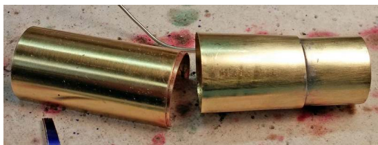
Figure 98: Here the last boiler section waits to be soldered into place. This last seam was soldered from the inside of the boiler.
