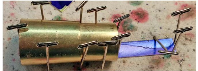
Figure 95: The seams for both the smoke box and the sloped boiler section are on the bottom. Those seams were soldered on the inside of the tubes, which is a preferable technique whenever feasible.
