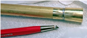
Figure 96: A fiberglass mini brush (Micro-Mark #14259) is a good tool for cleaning excess solder from a joint.
