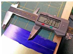
Figure 87: A sheet of 0.010 inch brass was scribed 0.6420 inches from one end and then marked for the length of the smokebox circumference. This was calculated by using D = C , thus 0.6420" \times 3.1416 = 2.017" inches.
