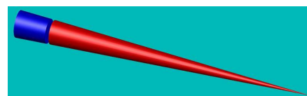
Figure 91: The blue portion of this simple rendering is the section of this oblique cone which will eventually become part of the wagon top boiler for Shay #6.
