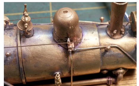
Figure 152: A piece of 0.008 brass rod was used to make the sand release control cables. A #80 bit was used to drill pass through holes in the cab front for these. Both control cables were bent by hand into a drooping shape and then soldered to the levers and the cab front.
