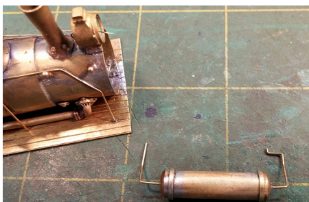
Figure 153: Here the plumbing to and from the air reservoir are shown bent into shape and cut to fit under the Shay's boiler.
