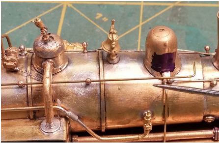
Figure 147: As so often done in the past I used Dykem on the sand dome and scribed mark using the brass rod in the original two stanchions as a guide.
