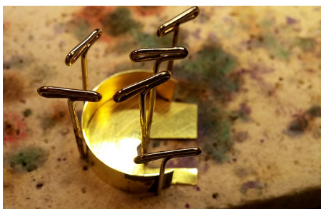
Figure 157: The brass strip was placed around the outside of the backhead plate so that it might fit around the rear end of the boiler.
