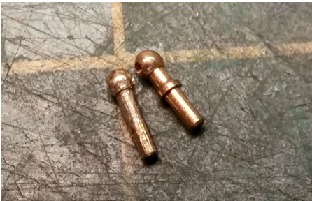
Figure 149: The modified stanchion is, obviously, on the left. The entire length of the shaft had to be the diameter of the mounting stud.
