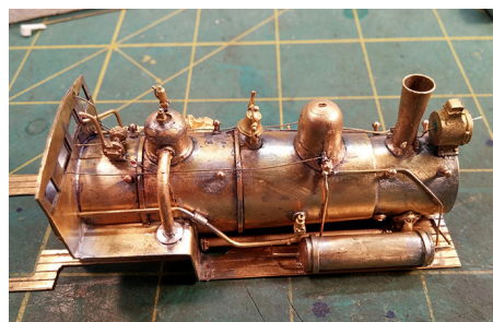
Figure 154: The air reservoir shown after attaching it to the deck using a flat head 1-72 screw. The hole in the tank was piloted with a #76 drill and then taken to its full diameter with a #53 bit before tapping. Note: the sand release cables can be seen in this photo.
