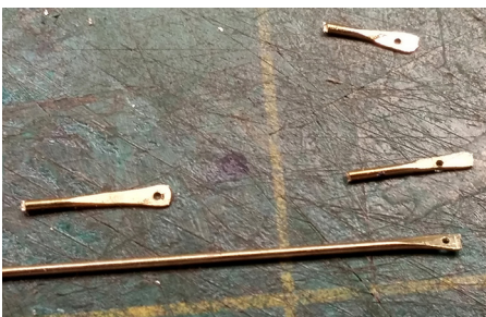
Figure 151: It took several tries to achieve a shape that I was happy with for the sand release levers on my Shay #6. The one at the bottom of the picture is the one I used. The holes were drilled with a #80 bit.
